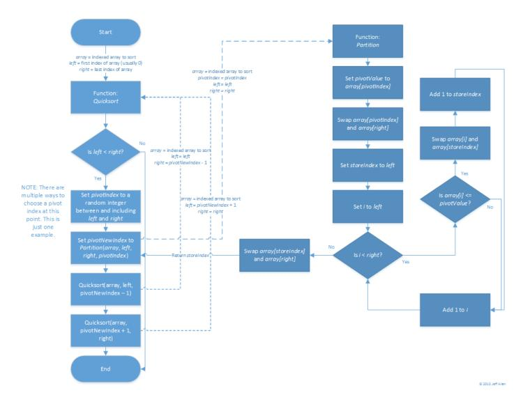
**QuickSort** is a Divide and Conquer algorithm. It picks an element as pivot and partitions the given array around the picked pivot. There are many different versions of quickSort that pick pivot in different ways. Always pick first element as pivot, Always pick last element as pivot (implemented below), Pick a random element as pivot, Pick median as pivot.
